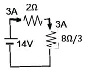
Thus the total resistance is  $R_{\rm tot}=2\,\Omega+8\,\Omega/3=14\,\Omega/3=4.67\,\Omega$
